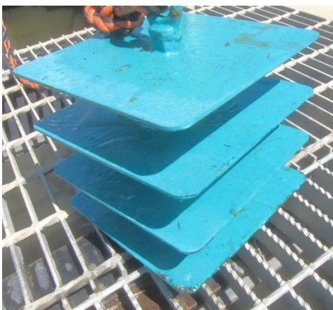
Paint-coated settling plates
